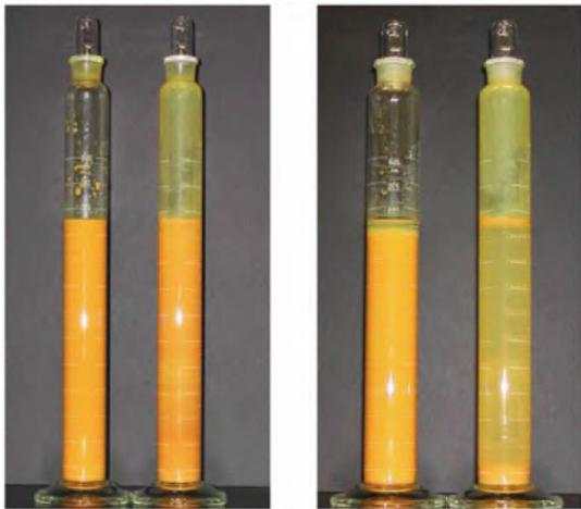
Each cylinder above contains 1 gram of iron oxide and 200mL of deionized water. The cylinder on the LEFT in both photos contains 100ppm of BW. Each cylinder was shaken 100 times and left undisturbed for 24hrs (picture on the right). The solution with BW was able to suspend the powders while also limiting residue re-deposition on the glassware.
